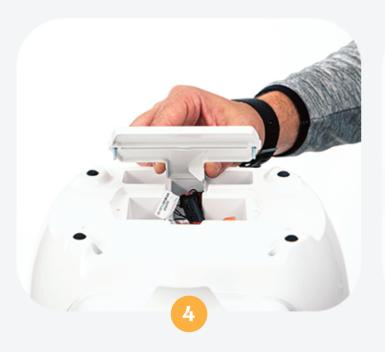
Connect the battery, making sure to connect the leads and terminals correctly: RED lead to the RED terminal and BLACK lead to the BLACK terminal.
