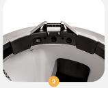
Snap the front of the bracket forward to secure it onto the bezel. (You will hear a snap.) NOTE: Ensure the bracket is positioned above (not obstructing the lasers) and is centered on
