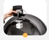
Place the bundle of wire in the wire cover pocket and route the wire attached to the camera end through the slot. NOTE: Keep the bundle of wire as low as possible in the wire cover pocket to avoid interference with
