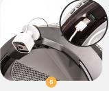
Mount your camera to the hinge and plug it into the USB port behind the control panel. NOTE: The camera mount has many different configurations. Now would be a good time to check your desired camera angle. You can adjust the angle by flipping the hinge, flipping the side the magnet is on, or flipping the camera. Be careful not to pinch your fingers!
