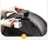
While keeping the wire in the wire cover pocket, snap the wire cover onto the bracket using the slots provided. (Be careful not to dislodge the bracket from the bezel at this step.) NOTE: Ensure the wire cover sits cleanly on the bezel. If It does not, the wire may come loose from the wire cover pocket and interfere with the bezel.
