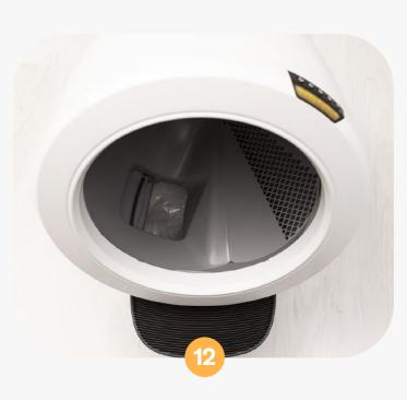
Observe two clean cycles to ensure the new seal strips don't get pulled up. Watch as the dump port rotates over the waste port area—if the seals are not adhered well enough, they could get pulled up by the rotating globe and cause an over-torque fault or a globe position fault. Reference this video for further information.
