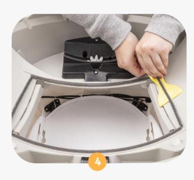
✓ Locate the old upper waste port seal strips in the base. Use a putty knife, flathead screwdriver, or your fingernail to lift the corner of a strip and peel off all four (4) strips.
