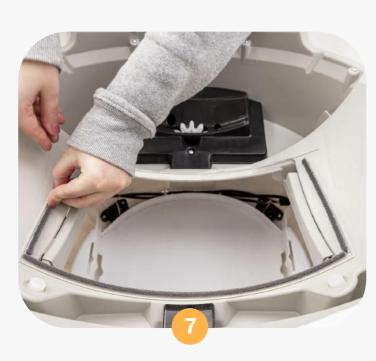
Next, replace the (2) side seal strips, which are 6"L. Place immediately adjacent to the forward seal strip, and along the inside of the strip guideline.
