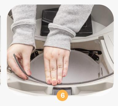
Replace the forward seal strip first, which is 13.5"L. Peel off the adhesive backing on the strip and place it along the inside of the strip guideline. Run your finger along the strip a few times to ensure adhesion.
